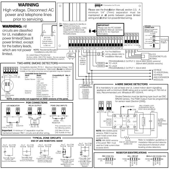
WARNING- Not to be removed by anyone except occupant: This equipment should be installed in accordance with the ANSI/NFPA 72 (National Fire Protection Association, Batterymarch Park, Quincy MA, 02269). Printed information describing proper installation, operation, testing, maintenance, evacuation planning, and repair service is to be provided with this equipment. For compliance with UL-985, at least one hard-wired smoke detector is required.
